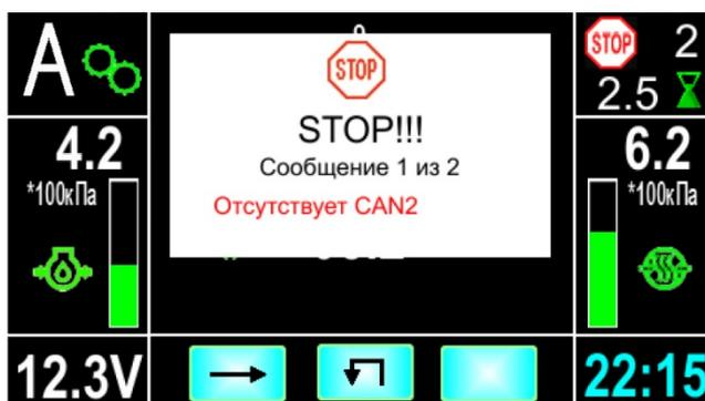
Figure 2.23.10 – Example of critical failure display
