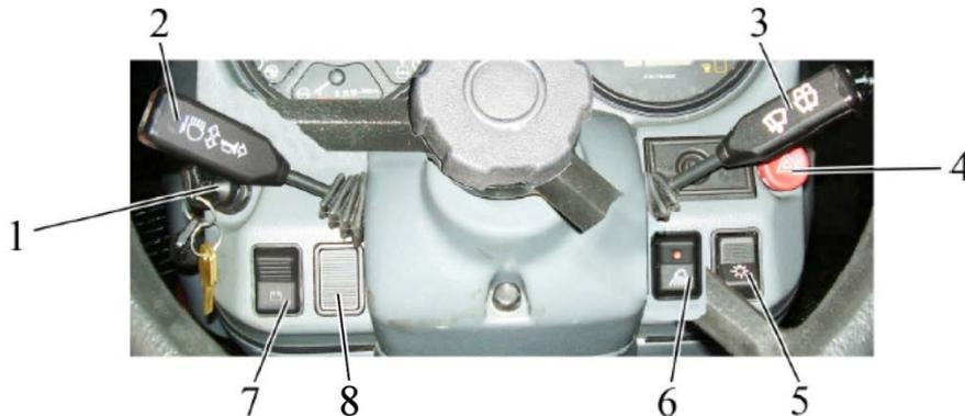
1 – starter and instruments disconnect switch; 2 – left multifunctional steering column switch; 3 – right multifunctional steering column switch; 4 – emergency flashing switch; 5 – central light switch; 6 – switch of front working lights mounted on front lights brackets; 7 – accumulator battery remote disconnect switch, 8 – blind plug.
